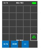
1. Navigate through pages of the "main screen" and select desired white-listed cell. Upon selecting, option buttons **«B/W»** and **«ROM»** will appear at the bottom of the screen.
