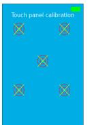
Touch panel calibration can be done with a stylus (included in the set), by pressing the center of the targets that will appear in different parts of the screen.
