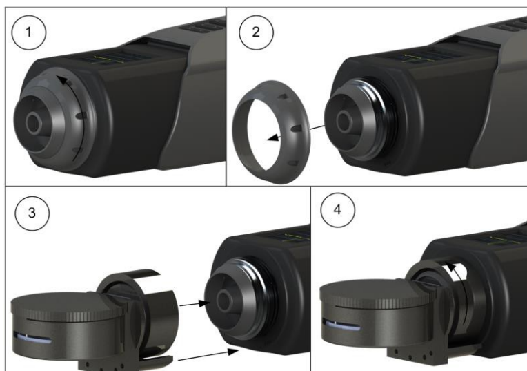
Figure 24. Piezo desorber connection procedure.
